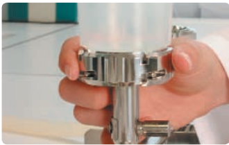
(A) Tight sealing of funnel and membrane reducing any cross contamination to a minimum by special sealing technique.
