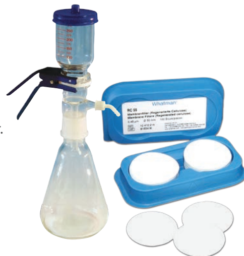
Whatman RC55 filters and GV 050/2 vacuum filtration unit.
