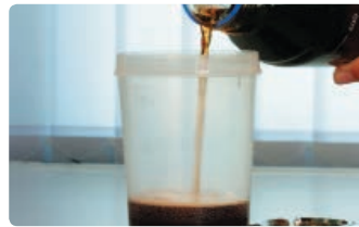
(B) Apply liquid and allow to filter through.
