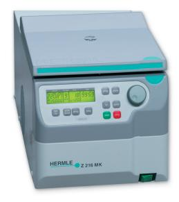
Universal Centrifuge Z216 -M Max. speed 15,000 rpm Max. volume 44 x 1.5 / 2.0 ml
